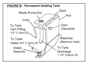
4. Turn discharge fitting of toilet to face intake of tank and connect using sanitation hose (#CHTT8), provided. Secure ends with hose clamps.
