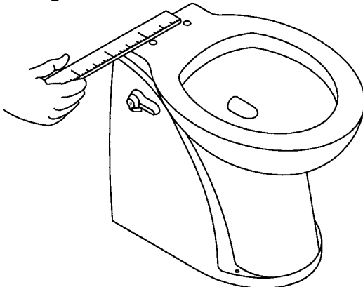
Figure #2 Center-to-Center Distance of Seat Mounting Holes
