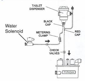
Developed at the request of Crown Head owners, the PURASAN is ideal for use with any of Raritan's macerating toilets in fresh water applications. A single tablet cartridge is placed in the tablet dispenser and lasts for several hundred treatment cycles.
