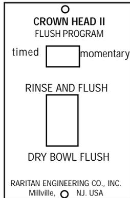
The crown head II optional deluxe control allows for selection of timed or momentary operation. Rinse and Flush provides normal operation, Dry Bowl Flush allows evacuation without drawing in additional water.
