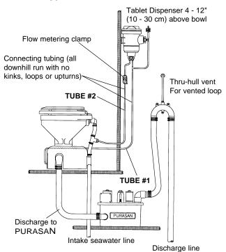
Developed at the request of Crown Head owners, the PURASAN is ideal for use with any of Raritan's macerating toilets in fresh water applications. A single tablet cartridge is placed in the tablet dispenser and lasts for several hundred treatment cycles.
